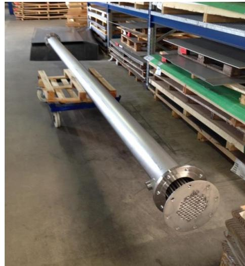
Abb. 21: Kondensator
