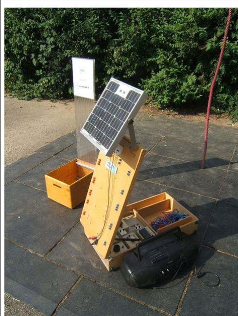
Abb. 3 Station 1 Photovoltaik-Koffer
